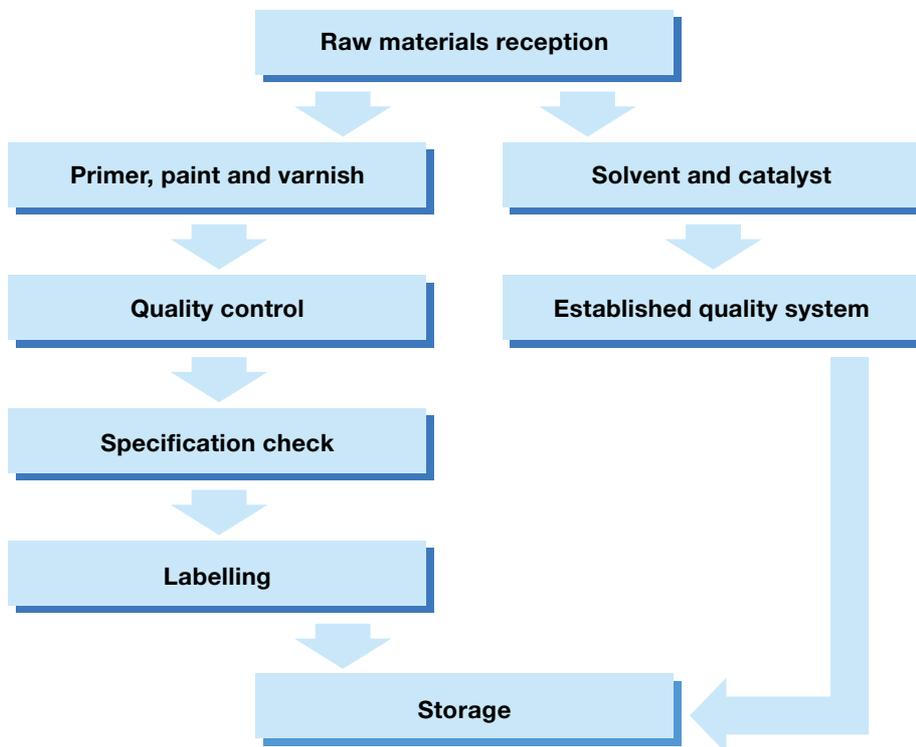
The paint pots come in one at a time and are stored in containers-prefab modules measuring 40 m<sup>3</sup>, as described in the corresponding section, opposite the paint entrance to the manufacturing shop. These containers, as mentioned previously, are equipped to maintain the paint at the right temperature. If the paint pots are small or a lot arrive at once, they come shrink-wrapped on pallets.
